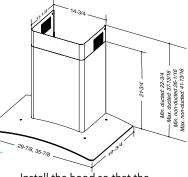
Install the hood so that the bottom of the unit is 24" to 30" above the cooking surface. Mounting height may be affected by ceiling height.
