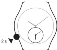
**1b.** Immediately slide your finger along the right hand side of the case from top to bottom. The minute hand moves slightly from right to left and the watch emits a small beep.
