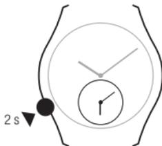
**1b.** Immediately slide your finger along the right hand side of the case from top to bottom. The same minute hand moves slightly again and the watch emits a small beep.
