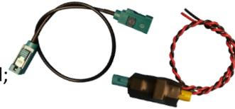
3. Connect the **red wire** from the GPS-Break board to the **white/blue, OUTPUT (A)** wire from the 18-pin **SRX VIM** module harness. Splice the **black wire** from the GPS-Break board to ground.
