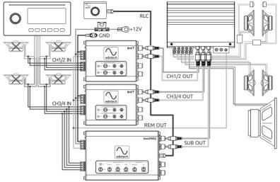
Note: Multiple linkTs can be used for aligning more channels such as front and rear, biamped components, or large subwoofer systems. Other Wävtech models can also be added for additional conversion channels and features. In this example, the bassFREQ provides remote level control, parametric EO and -24dB/oct crossover for a subwoofer.
