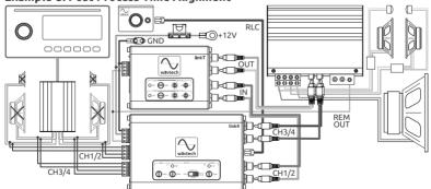
Note: When adding the linkT for time alignment after another Wavtech model such as the link4, adjust the link4's gain to both maximize the linkT's input signal without clipping and match its output with the input capability of the connected amplifier(s).
