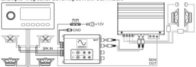
Note: When using a receiver's internal power IC to drive speakers directly and provide the linkT with signal, note that its speaker outputs will likely clip below the maximum master volume level. Adjust gain settings accordingly for optimum unclipped volume range.
