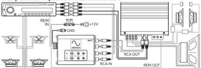
Note: When adding time alignment only for front speakers and retaining deck power to rear speakers, it is recommended to use the fader to reduce rear speaker level enough to provide some ambience while minimizing any affect to front staging and image focus.
