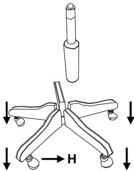
1. Insert the Pneumatic Cylinder into the base, this is a taper fit no mechanical fastening is necessary.
