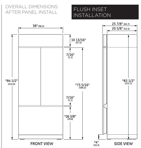
\* Shipping height. Use leveling legs and wheels for maximum 1" height adjustment from shipping height.
