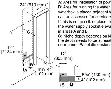
**A**: Area for installation of power connection.
