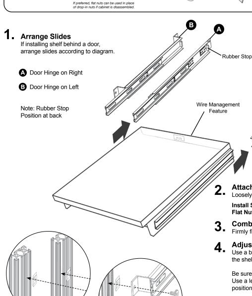
Attach Slides to Frame Loosely assemble hardware to slides as shown.
