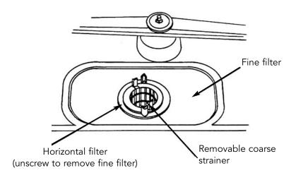
**WARNING:** Never operate the dishwasher without the filters in place.
