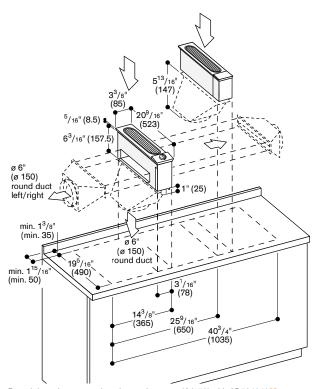
Round duct pipe connection piece to bottom ø 6" (150) with AD724040\*\* Round duct pipe connection piece to left/right ø 6" (150) with AD724040\*\* + AD724041
