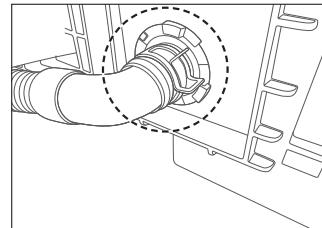
Tighten the clamp in the center of the assembly position.
