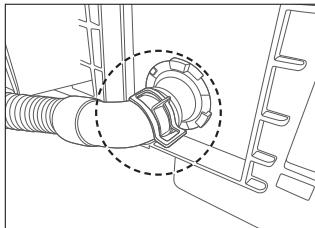
The clamp is improperly connected.
