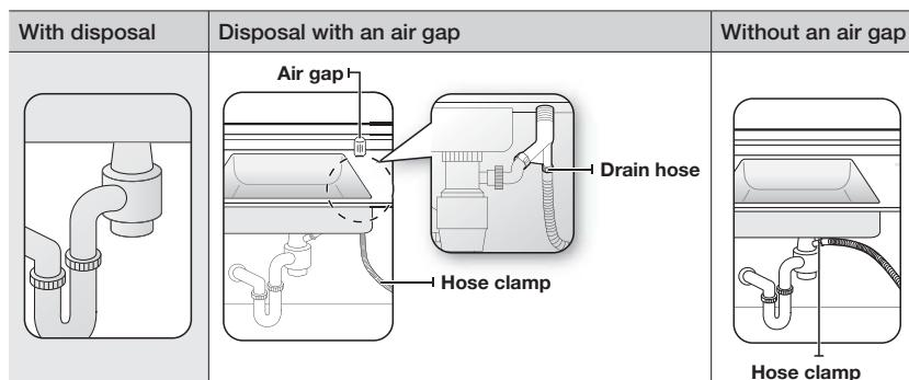
3. Check the size of the sink's drain hose connector. If needed, cut the drain hose so its end fits onto the sink connector ( $\frac{1}{2}$  in.,  $\frac{3}{4}$  in. or 1 in. - as shown in Figure 11 below). If the end of the drain hose does not fit onto the drain hose connector of the sink, use an adaptor purchasable at a plumbing/hardware supply store.
