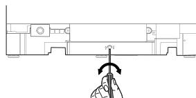
Before you move the dishwasher for installation, make sure to adjust the height of the legs so the legs are as short as possible. This prevents the legs from breaking. Level the dishwasher by adjusting the height of the legs after you have the dishwasher in place.
