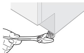
To adjust the height of a rear leg, turn the Hexbolt (at the front of the base) to the left to raise the back of the dishwasher using the proper tool (Hex L-wrench or similar tool).
