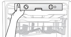
2. Use the level to check if the dishwasher is level front to back, as shown in the figure to the right. If the dishwasher is not level front to back, adjust the height of the rear leg until the dishwasher is level. See the second note below for instructions on adjusting the the rear leg.
