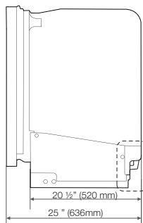
The water supply line, power cable and drain hose should go through this space behind the dishwasher. Then, they run in channels under the dishwasher to connections in the front.
