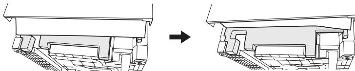
6. Confirm that the kick plate gasket is on the bottom of the kick plate. To install the kick plate, refer to the figure below.
