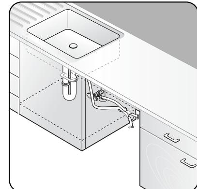
The hole for the water supply line, drain hose and power cables.
