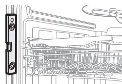
3. Open the door of the dishwasher and check if both the tub and door clearances are correct. If not, rotate the leveling legs on the bottom front of the dishwasher. You can also check this by placing a level against an inside front vertical surface of the tub.
