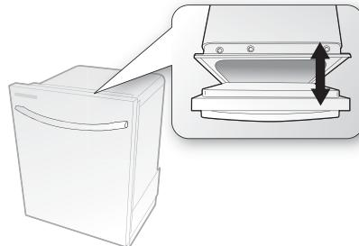
If the leveling legs are rotated to the right (counter clockwise), they are loosened and the front of the dishwasher is raised. If they are rotated to the left (clockwise), they are tightened and the front of the dishwasher is lowered.
