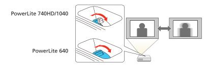
If your image looks like \_\_\_\_ or \_\_\_\_, you've placed the projector off to one side of the screen at an angle. Place the projector directly in front of the center of the screen, facing the screen squarely. If you can't move the projector, use the horizontal keystone slider on the projector to correct the image.
