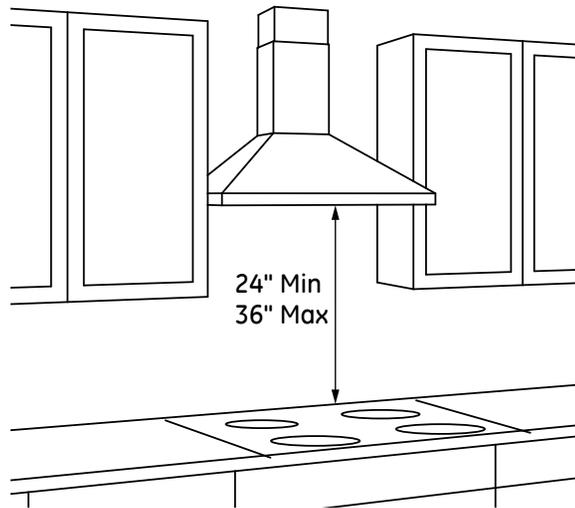
The vent hood must be installed 24" min. and 36" max. above the cooking surface. The hood installation height above the cooking surface depends upon ceiling height. The telescopic duct cover conceals the ductwork running from the top of the hood to the ceiling.
