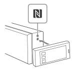
Follow the on-screen instructions displayed on the remote device, and complete the procedure for BLUETOOTH connection. When the BLUETOOTH connection is established, the blue LED indicator on the front panel lights
