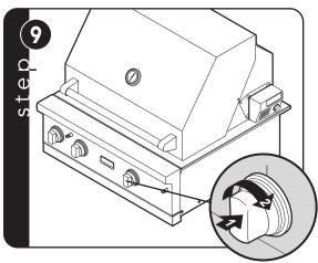
After checking for leaks, push in and turn any control knob to release the pressure in the hose and manifold.
