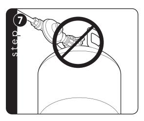
Do not attempt to repair the cylinder valve if it should become damaged. The cylinder must be replaced.
