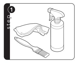
Make a soap solution of one part liquid detergent and one part water. You will need a spray bottle, brush or towel to apply the solution to the fittings.
