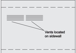
An enclosure for an LP-gas cylinder shall be ventilated by openings at both the upper and lower levels of the enclosure. The effectiveness of the opening(s) for purposes of ventilation shall be determined with the LP-gas supply cylinder in place. This shall be accompanied by one of the following:
