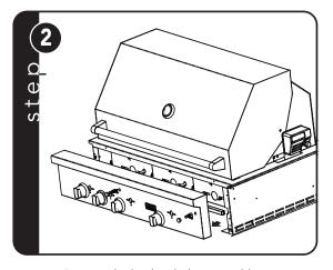
Remove the landing ledge assembly. **Note:** Leave wires connected to switches on valve panel.
