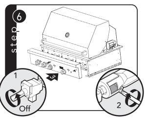
When adjustments are complete, turn the valve off, tighten the air shutter screw, and replace the landing ledge assembly
