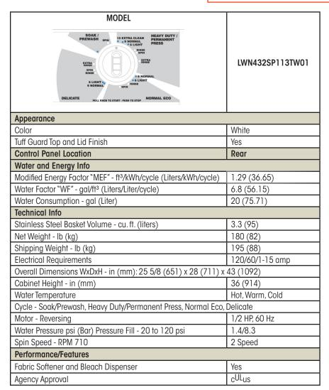
For the most accurate information, the installation guide should be used for all design and construction purposes. Due to continuous product improvements, design and specifications subject to change without notice. The quality management system of Alliance Laundry Systems' Ripon facility has been registered to ISO9001:2008.
