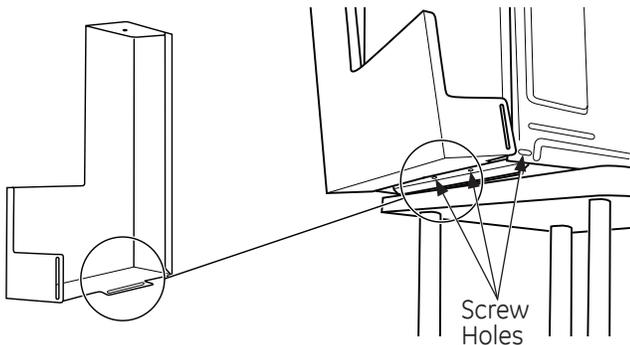
5. Your microwave will have one or two screws on the bottom left side. Remove these screws to create a gap between the bottom plate and the case of the microwave.
