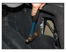
**S T E P 1 0**Reinstall the trunk liner. Using a hammer, lightly tap the position of the 3/8 - 16 x 2-1/4" Set Screw to mark the inside of the trunk liner.
