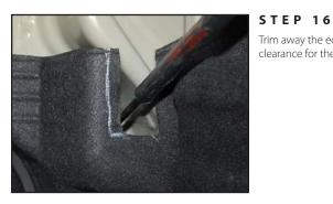
Trim away the edge of the trunk liner as indicated to allow clearance for the shock.
