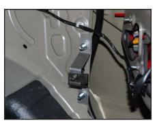
**STEP 9**Pictured is the Bracket attached to the brace.
