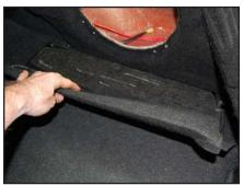
**STEP 15**Fold and tuck the remaining floor carpet under the Stealthbox®.
