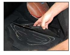
Peel the carpet away from the flap on passenger side of the trunk floor.
