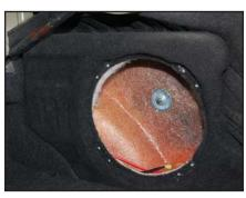
Using a Phillips head screwdriver, remove the subwoofer from the Stealthbox®. Connect speaker cable to the terminals on the enclosure, and put the enclosure into position, allowing the 3/8 - 16 x 2-1/4" Set Screw to pass through the hole in the back of the box. Slide a 3/8" Fender Washer, a 3/8" Flat Washer, a 3/8" Lock Washer, and a 3/8 - 16 Hex Nut over the 3/8 - 16 x 2-1/4" Set Screw, and firmly tighten. Route the speaker cable as necessary.
