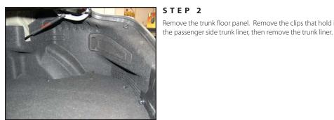
STEP 2 Remove the trunk floor panel. Remove the clips that hold in
