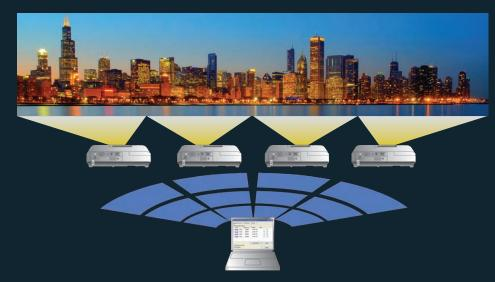
You can use either wired or high security wireless LAN connections and project the same or up to four different images on up to four projectors, or display a panoramic image.
