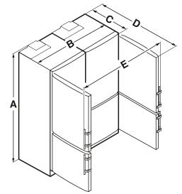
Overall height can be increased on CS 14 and all CS 16 units by 5/8" (16 mm).
