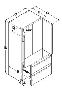
Overall height can be increased on CS 20 units by 1-1/2" (40 mm).
