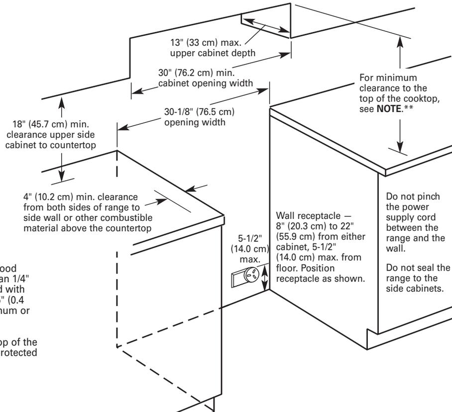
**\*NOTE:** 24" (61 cm) min. when bottom of wood or metal cabinet is protected by not less than 1/4" (6.4 mm) flame retardant millboard covered with not less than No. 28 MSG sheet steel, 0.015" (0.4 mm) stainless steel, 0.024" (0.6 mm) aluminum or 0.020" (0.5 mm) copper.
