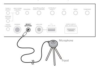
If you have a tripod, use it to place the microphone so that it's about ear level at your normal listening position. If you do not have a tripod, use some other object to install the microphone.
