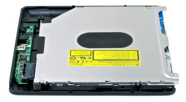
Slide the drive mechanism through the front opening of the bottom case until it the drive is fully inserted into the bridge card and is flush with the front of the drive opening.
