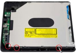
On the back and side of the enclosure you will see 3 cutouts for screws to be inserted into the optical drive mechanism. Secure the optical drive mechanism to the bottom case with the included Phillips collared screws.
