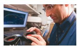
The profile of the ear-pads is as smooth as possible to reduce wrinkles that in turn cause leakage and loss of insulation.
