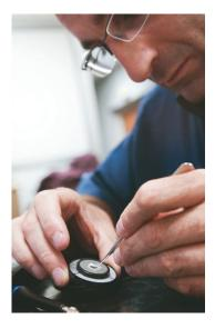
The choice of capsule is an essential element that determines the sound quality of the headphone. Every mylar / titanium 40mm capsule used in the manufacture of the Spirit One headphone is systematically measured and tested to ensure utmost reliability in its performance and reproduction of sound.
