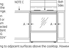
. This appliance has been approved for 0" spacing to adjacent surfaces above the cooktop. However, a 6" (15.24cm) minimum spacing to surfaces less than 15" (38.1cm) above the cooktop and adjacent cabinet is recommended to reduce exposure to steam, grease splatter and heat.
