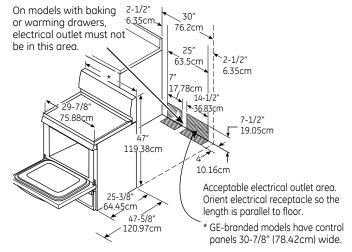
NOTE: Use a 4' (1.22m) power cord to prevent interference with the storage drawer. Power cords 4-1/2' (1.37m) to 6' (1.83m) long may have to be dressed to allow for proper drawer closing.
