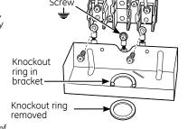
**NOTE:** Do not install the power cord without a strain relief. The strain relief bracket MUST be installed before reinstalling the rear range wiring cover
