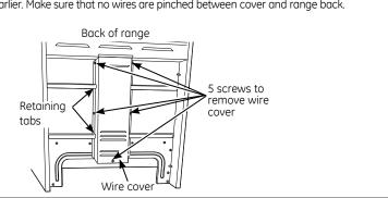
7 ANTI-TIP DEVICE INSTALLATION
