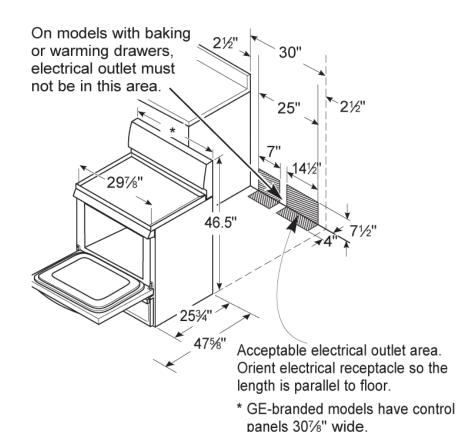
**NOTE:** Use a 4' power cord to prevent interference with the storage drawer. Power cords  $4\frac{1}{2}$ ' to 6' long may have to be dressed to allow for proper drawer closing.
