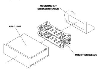
TYPICAL FRONT-LOAD DIN MOUNTING METHOD
