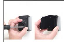
Place the Tilt Swivel base plate over the matching holes in your mounting bracket (demo ProClip mount shown in picture) Attach the base plate by using the applicable screws enclosed self-tapping screws if the mount has small holes or machine screws with nuts if the mount is made of metal and has large holes. Place the holder onto the base plate.
