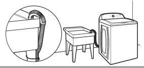
Minimum capacity: 20 gal. (76 L). Top of laundry tub must be at least 39" (990 mm) above floor; install no higher than 96" (2.44 m) from bottom of washer.
