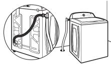
Floor drain system requires additional parts. Minimum siphon break: 28" (710 mm) from bottom of washer.
