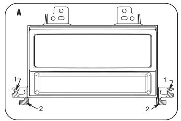
Mount the ISO Brackets to the head 2 unit with the screws supplied with the unit. (Figure B)
