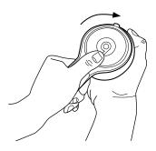
**Cushion reattachment:** Special attention needs to be paid to alignment of the three clips on the inside of the cushion and the earcup as well as the notch on the bottom of the cushion. It will be extremely helpful to examine the three clips inside of the cushion and on the earcup and note how they fit together before reattaching the cushions.
