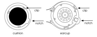
Grip the headband and cushion as described in the removal section. Aligning the clips on the cushion and the earcup, place the cushion firmly against the earcup with the notch on the bottom of the cushion to the left of the headphone cable port. With your thumb firmly pressed against the "b" logo, simultaneously press the cushion and earcup into each other and twist the cushion counter clockwise. The cushion should be attached firmly, with all three clips engaged.
