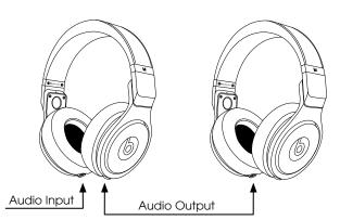
**Note:** No switching is needed. The Dual/Input Output functionality works automatically and is not dependent on which of the two Beats<sup>w</sup> Pro ports, left or right, is connected to your audio gear's output port. Either side can work as an input or output.
