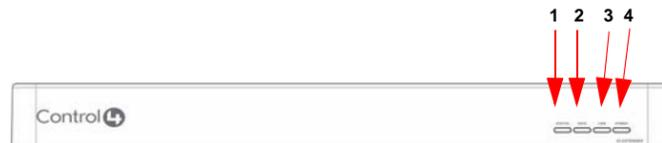
1. **Status LED**—Red, Orange and Blue blinking lights indicate the status during startup.
