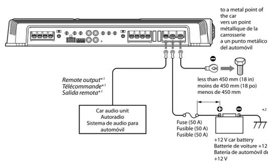
\* If you have the factory original or some other car audio unit without a remote output for the amplifier, connect the remote input terminal (REMOTE) to the accessory power supply.
