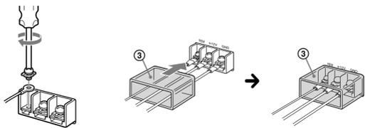
Pass the wires through the cap, connect the wires, then cover the terminals with the cap.
