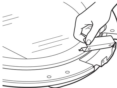
Place the door on its edge and secure the window retainer using the 2 machine screws (#8).
