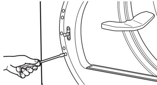
Switch the strike bracket and its cover on the opposite side by removing the screws. Reinstall both on the opposite side.
