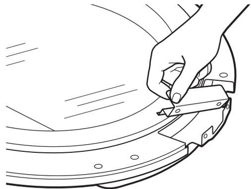
Remove the hinge assembly by removing the 2 machine screws (#8) that fasten it to the frame. Pull the hinge assembly out of its cavity and set it aside.
