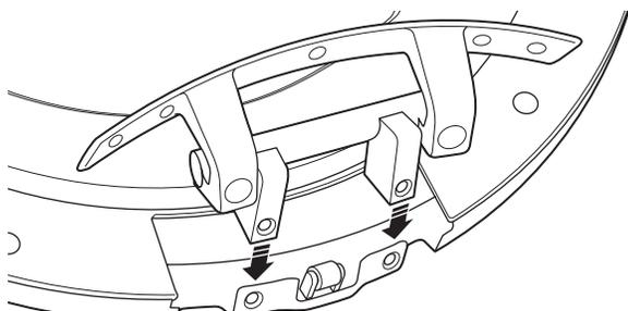
Fasten the hinge assembly to the edge using 2 machine screws (#8).
