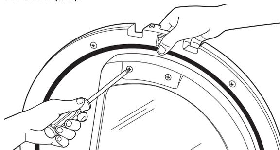
Insert the hinge cover. Align the hinge cover holes with the holes in the door.
