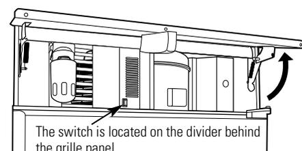
The switch is located on the divider behind the grille panel.
