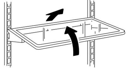
**To replace shelves:** Select desired shelf height. With shelf front raised slightly, engage top lugs in tracks at rear of cabinet. Then lower front of shelf until it locks into position.
