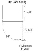
• The door swing is reversible on all models. If desired, change the door swing before installation.
