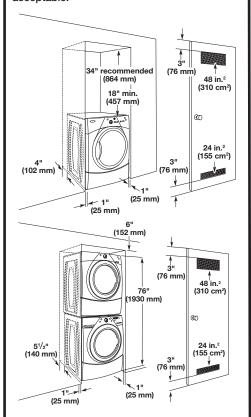
For cabinet installation, with a door, the minimum ventilation openings in the top are required.
