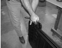
**STEP 4:** Using a 3/8" drive ratchet and a T-30 Torx socket. Remove the pair of latches from the mid-gate.
