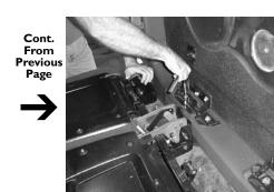
**STEP 7:** With help from a second person, place the Stealthbox into the vehicle and into position.
