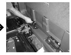
**STEP 2:** With a 3/8" drive ratchet and a 13mm deep socket. Remove the bolts and nuts that secure the hinges to the mid-gate and floor.
