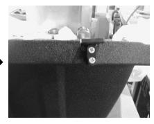
**STEP 5:** Mount the OEM latches to the top of the Stealthbox. Using the supplied four(pair per latch) phillips head screws and also using the OEM spacer per screw.
