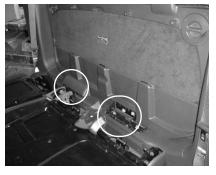
**STEP I:** With the front seats moved as far forward as possible and the rear seats folded down. Remove the pair of plastic hinge covers.
