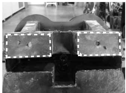
STEP 7 Turn the bottom section of the storage console, to expose the bottom side. Mark the two areas shown in the picture. With a cut off wheel or similar tool, cut out these two sections.
