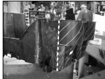
STEP 11 Ending at the front right of the storage console. Mark the line shown in the picture, top to bottom. With a cut off wheel or similar tool, cut on the marked lines from STEPS 9-11 .
