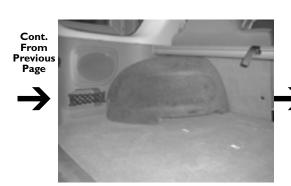
**STEP8:** With the socket cup set screw still threaded in the Stealthbox, place the Stealthbox into place.
