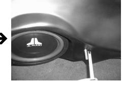
**STEP 4:** With the wax square properly placed, thread the supplied socket cup set screw into the Stealthbox. Leaving about 1.5" exposed. Place Stealthbox in installation area and press down.
