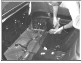
STEP 13: Place "Unuts" (supplied)through the stamped factory holes and over the holes you have just drilled.
