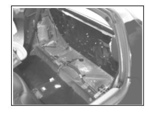
STEP 5: Unbolt and remove seat belt retractors from both sides of the car (two bolts per retractor).
