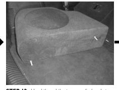
**STEP 12:** Hand thread the two supplied socket cup set screws into the bottom of the Stealthbox, leaving about 1" of each threaded rod exposed. Make sure that the slotted end is exposed.
