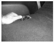
**STEP 5:** After the rivets are completely removed, the cleats should pull up. They are still going to be attached to the carpet.
