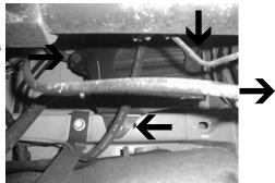
**STEP 13(b):** This is the more time consuming, but easier way to access the front exposed threaded rod. You need to unbolt the over flow gas can. Please make sure that you are careful and you do not tip over this plastic tank. Do not do this while smoking.
