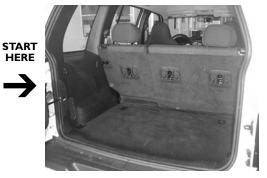
**STEP 1:** Open the rear door and remove any contents and the retractable security cover:
