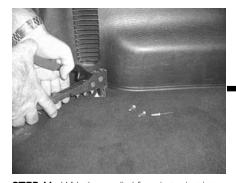
**STEP II:** With the supplied four rivets, rivet into the exposed holes from the drilled out OEM rivets from STEP?
