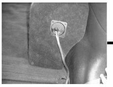
**STEP 15:** With the Stealthbox properly mounted, run speaker wire to the Stealthbox's terminal cup. Wire it up.
