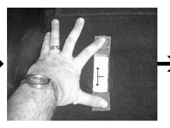
**STEP 8: Front Cleat Location:** Spread the carpet. Find the center between the two holes, then measure 1/2" out from the holes to the middle of vehicle. Then mark
