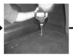
**STEP 9:** With 1/2" drill bit and drill. Drill at the marked locations from **STEP 7** & **STEP8**
