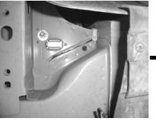
**STEP 14:** The rear exposed socket cup set screw is a lot easier to excess. Place a supplied 3/8" fender washer, a supplied 3/8" lock washer then a supplied 3/8" hex nut in this order onto the socket cup set screw. Thighten.
