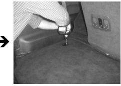
**STEP 4:** With a 1/4" drill bit, drill out the rivet's head. Then with a punch out and hammer, carfully tap out the rivet's body.
