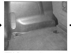
**STEP 2:** The enclsoure will be mounted on the driver's side cargo area. Both cleats are to be removed.
