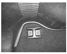
**STEP 3:** To remove both cleats, you need to remove both of the OEM rivets.
