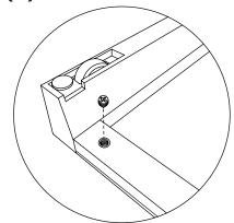
Place **Stretchers** so **Cams** are facing towards the wheels and the grooved edge detail faces outward.
