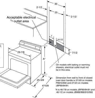
Dimension from wall to front of closed oven door handle is 27-3/4.
