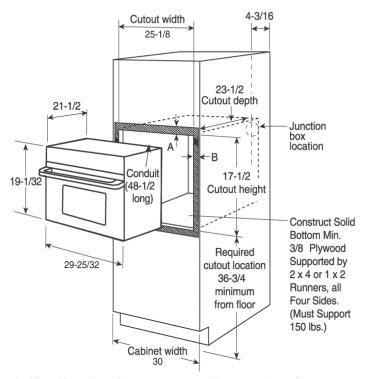
A=Allow 1" overlap of oven over top and bottom edges of cutout. B=Allow 11/16"-3/4" for overlap of oven over side edges of cutout.
