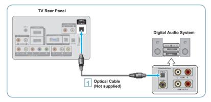
Connect an Optical Cable between the DIGITAL AUDIO OUT (OPTICAL) jacks on the TV and the Digital Audio Input jacks on the Digital Audio System.
