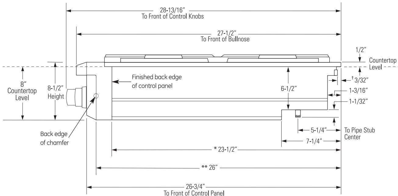
\* Minimum cabinet cutout depth from the back of the rear trim to the back finished edge of the control panel - typically, the minimum cabinet depth (front to back). Maximum cabinet cutout depth is 26" minus the countertop overhang.
