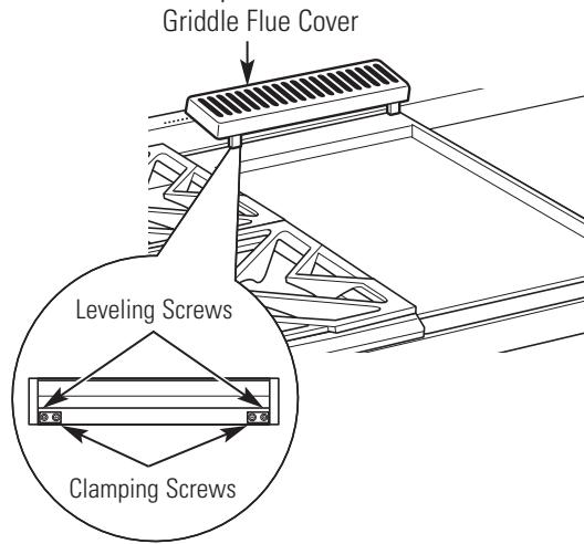
The two inner screws are clamping screws for securing the griddle in place. Loosen these two screws before leveling. Do not remove these two screws.
