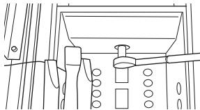
Reverse these steps to reassemble the griddle. Push excess capillary back into the entry hole. Place the unused orifice in the holder for possible future use.
