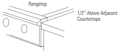
Front of deep cabinets can align with control panel beveled edge.
