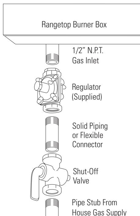
**IMPORTANT:** Disconnect the rangetop and the individual shut-off valve from the gas supply piping system during any pressure testing of that system at test pressures greater than 1/2 psig. Isolate the rangetop from the gas supply piping system by closing the individual manual shut-off valve to the rangetop during any pressure testing of the gas supply piping system at test pressures equal to or less than 1/2 psig.
