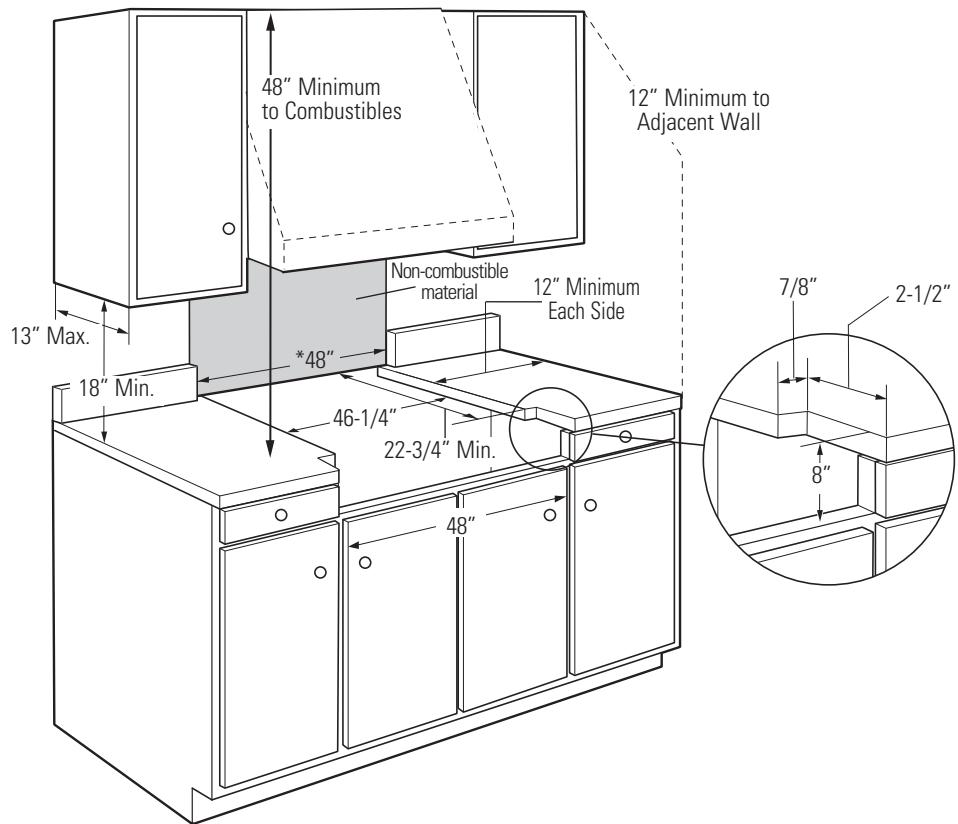
\* The opening between a 4" high backsplash must be 48" to allow the rangetop to slide back against the wall.
