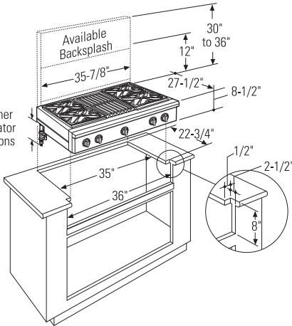
36" wide models are designed to fit in 36" or wider base cabinets
