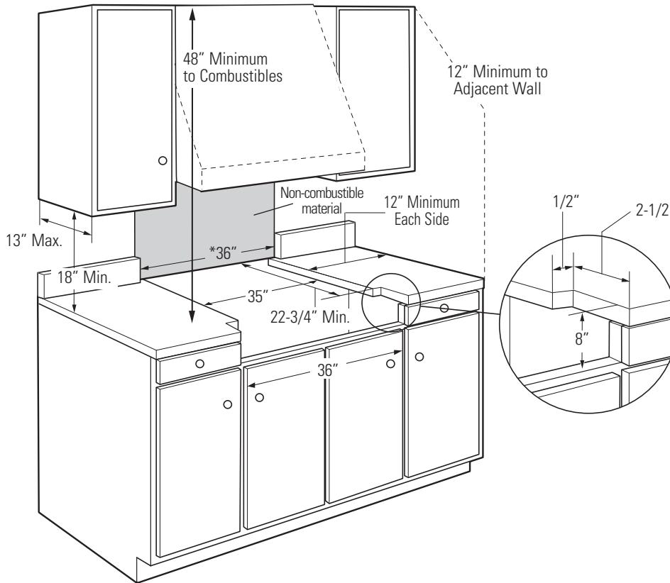
\* The opening between a 4" high backsplash must be 36" to allow the rangetop to slide back against the wall.
