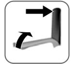
1. Lift lever + 2. push back as far as possible and hold for 3 seconds.
