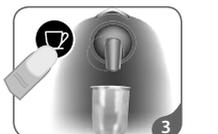
Press the (large) cup button and rinse by allowing a tank full of water to run through the coffee outlet.
