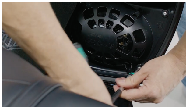
Fig. 2: Secure Grille With Silver Screws Using a T20.
