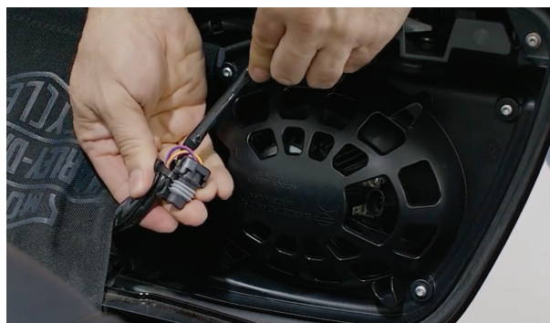
Fig. 3: Ziptie Tweeter Connector to Harness
