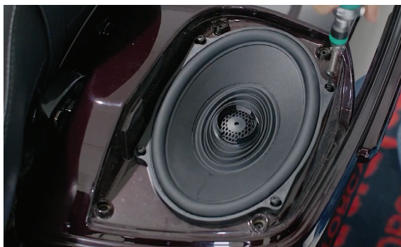
Fig. 1: Secure Speaker With Black Screws Using a T20
