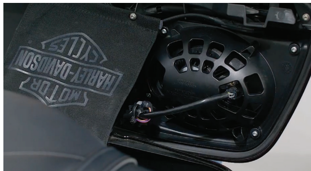
Fig. 4: Plug Main Harness Into TMS14-57
