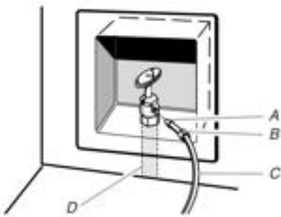
A. Bulb B. Nut C. Copper or PEX tubing (to refrigerator) D. Household supply line (1/2" minimum)
